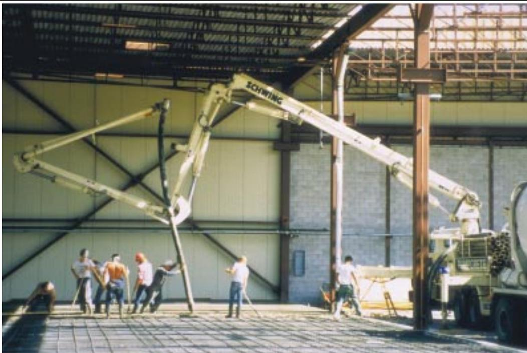
Front legs power out and down hydraulically. Rears easily extend manually and power down hydraulically to provide a stable platform for high volume pumping. Controls on both sides of the chassis add safety and speed to set-up. Convenient pad storage further enhances operator efficiency.
